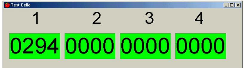
In case of problems on one or more lines, if there are doubtful on the weighting, it is with this function that the correct operation of the analogical section can be verified: cell of load, cables and amplifiers. The values that are read to empty and with a weight above, they have to be repetitive with a tolerance of some gram.
